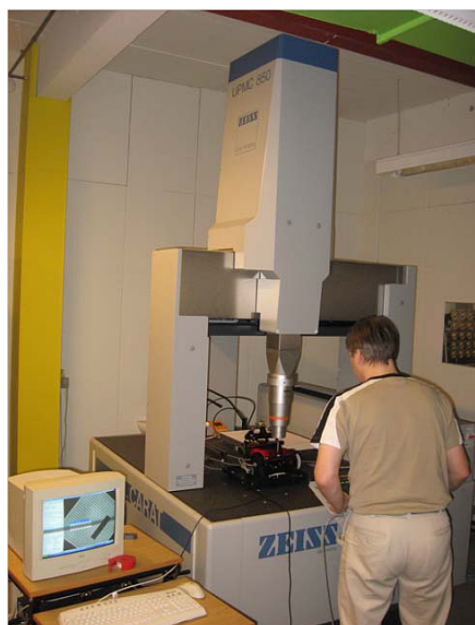
Figure 5: Left: Reference measurements with a high-end coordinate measurement machine (accuracy 3 microns). Right: Scan of an implant bar reference object with errors in the insertion direction [in microns].
